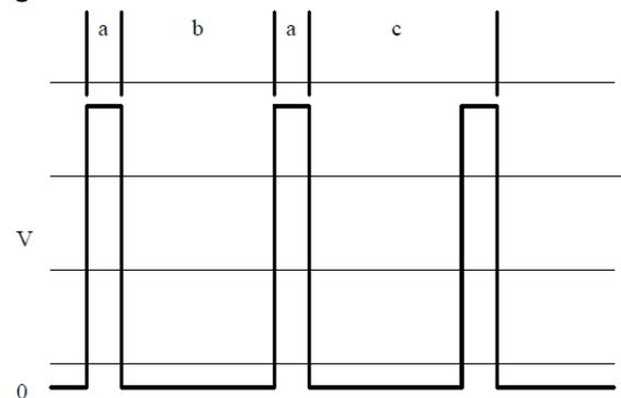
**Figure 2: Illustration of GroCelerator Concept.** The peaks (a) represent when voltage is flowing and valleys (b) represent when the circuit is open, using no electrical energy. The (c) space represents an entire on/off cycle.
